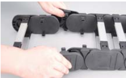
Line up two inner side links side by side. Attach an outer side link between
